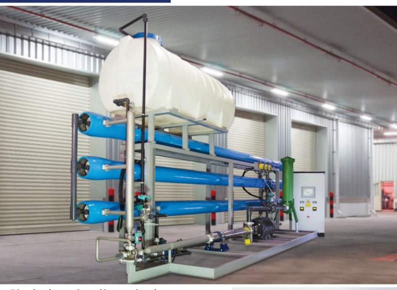
Dissolved organic and inorganic substances (bitter, high conductivity, etc salts, heavy metals, viruses and bacteria in the water are treated with reverse osmosis systems Up to 96 99 of purity in water could be achieved Water with different sources such as well water, tap water, sea water etc could be treated with high purity using Reverse Osmosis systems
