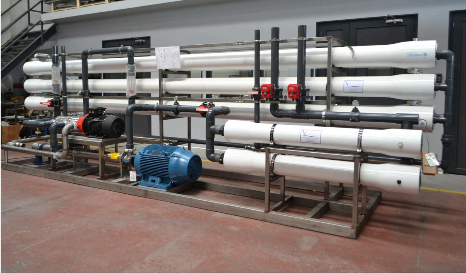
Dissolved organic and inorganic substances ( bitter, high conductivity, etc salts, heavy metals, viruses and bacteria in the water are treated with reverse osmosis systems Up to 96 99 of purity in water could be achieved Water with different sources such as well water, tap water, sea water etc could be treated with high purity using Reverse Osmosis systems
