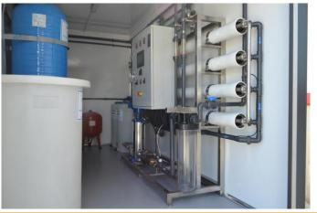
Trailer type water treatment systems are generally preferred at sites that have space problems and has less ability to have workforce. Specially, armies need Trailer Type Water Treatment System, because this Type Water Treatment is mobile and it has wheels.
